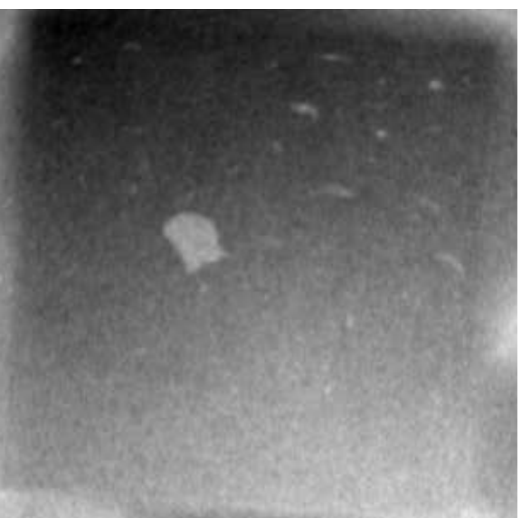
Figure 6. Typical solder attach taken from Au80/Sn20 solder batch.
