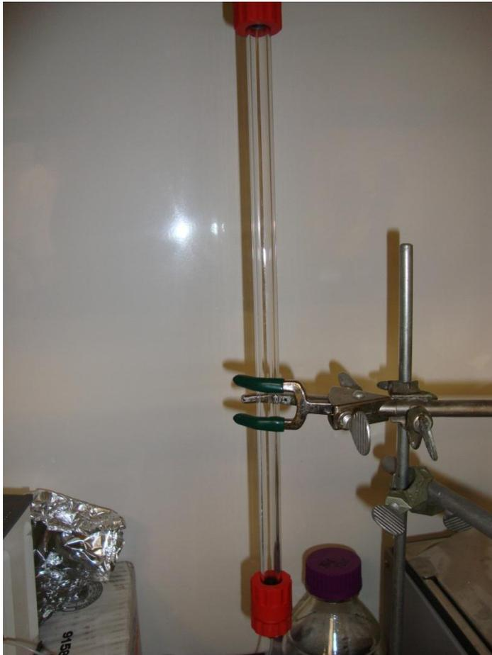
**Figure3.** Column used to separate excess and labeled protein.
