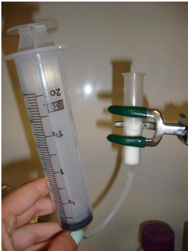
**Figure4.** The miniature column and syringe used to collect fractions.
