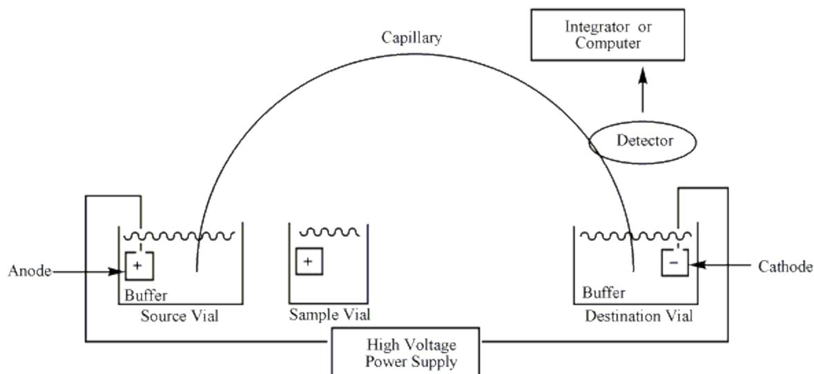
**Figure 1.** Diagram of the capillary electrophoresis process (8).
