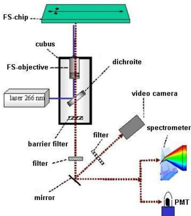
**Figure 2.** Diagram of the microchip electrophoresis process (9).
