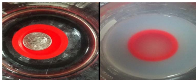
Figure 9. Comparison of treated water by UF (left) to the original feed solution (right) prior to treatment. Note: there is a quarter in both samples.
