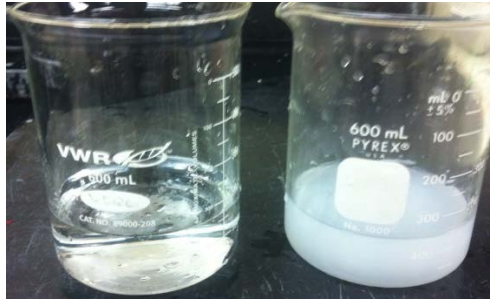
Figure 10. Comparison of UF-treated water (left) to the original feed solution (right) prior to treatment. Note: The samples in this picture are the same as those featured in figure 9, demonstrating that there was not a disproportionate depth of the two solutions.
