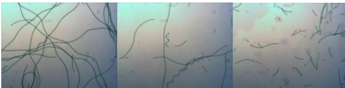
Figure 9. Hollow fiber membrane tangential flow filtration samples from left to right: before, single pass, multi pass.
