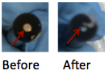
Figure 3. The platinum electrode before and after polymerization of EDOT. The red arrow points to the electrode surface.
