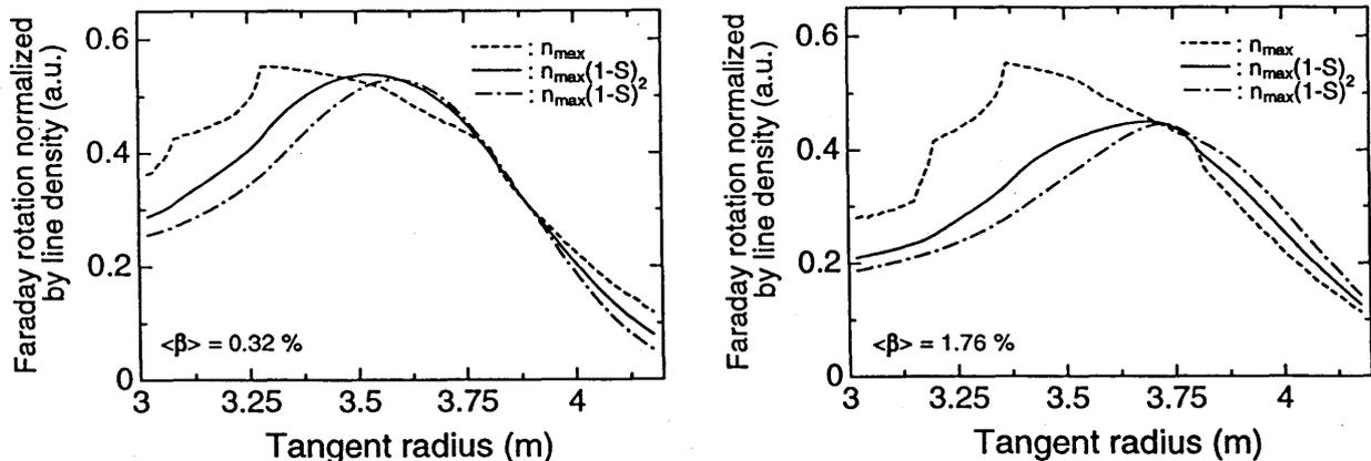
Fig. 1 Variation of the normalized Faraday rotation angle as a function of the tangent radius with three electron density profiles.
