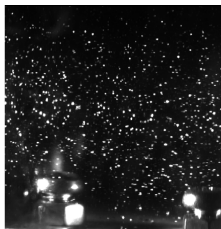
Figure 2 Tracer particles in liquid He at 1.6K.
