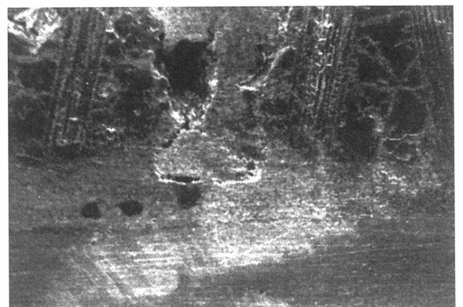
Fig.2 Microstructure of the joining part after heat load tests.
