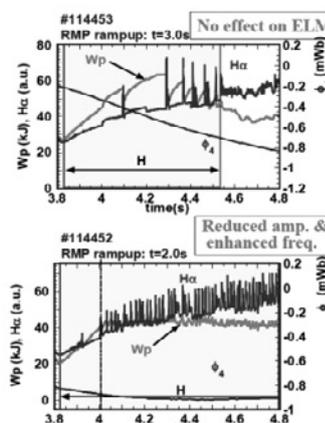
Fig.1 (a: upper traces) the case of late turn-on ( $t=3.0$  s) of the RMP pulse, (b: lower traces) the case of early turn-on ( $t=2.0$  s) of RMP pulse.
