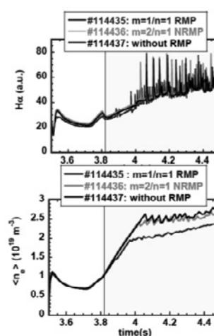
Fig.2 Comparison of three shots: #114435 with  $m=1/n=1$  RMPs, #114436 with  $m=2/n=1$  non-RMPs, and #114437 without both RMPs and non-RMPs.
