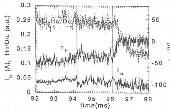
Fig.2 Time evolution of ion saturation current ( $I_{is}$ ) and floating potential ( $\phi_{fl}$ ) measured at  $\sim$ LCFS together with  $H\alpha/D\alpha$  emission, where a solid vertical line indicates the L-H transition and dotted line the pre transition.
