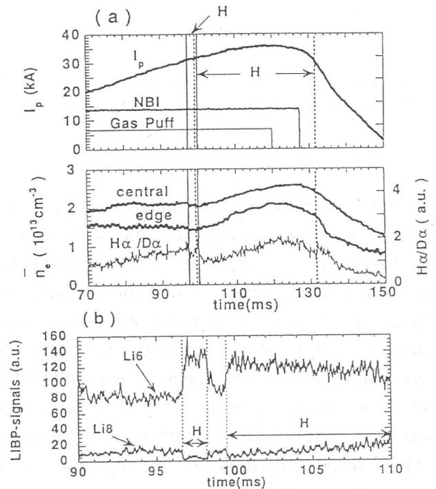
Fig.1 Time evolution of plasma parameters in a typical deuterium H-mode discharge.
