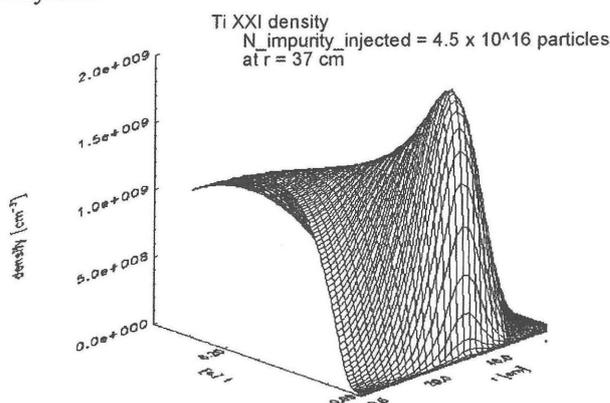
Fig. 3 Ti XXI density calculated by the MIST code.
