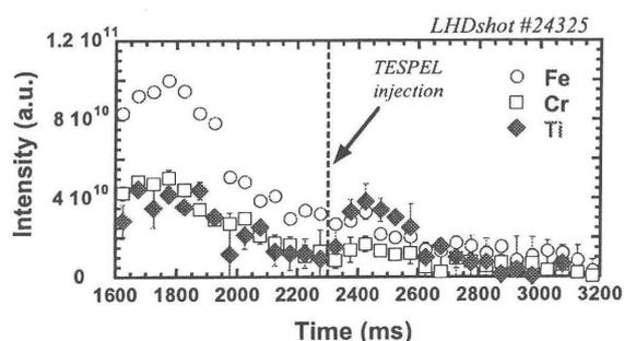
Fig. 2 Temporal evolution of the  $K\alpha$  line Intensity obtained by PHA system.
