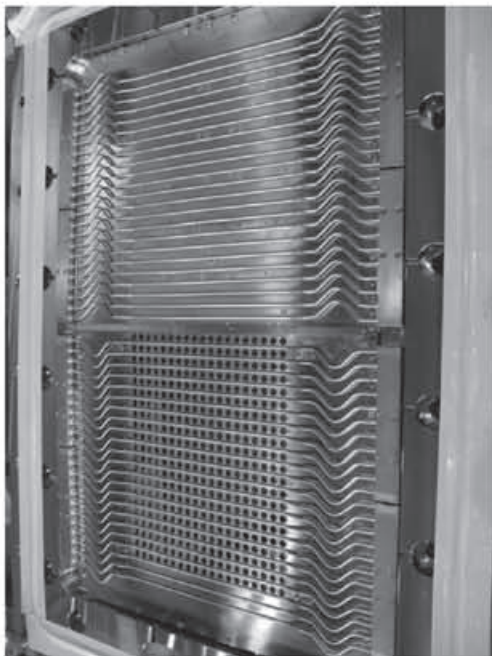
Fig. 1. Photograph of the plasma grid of the test positive-ion source. The lower half area is used for the beam extraction.
