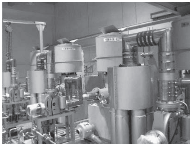
Fig. 1. Four 200 MHz transmitters and circulators transferred to the University of Tokyo from JAEA. Output power of 100 kW was achieved from each of the four transmitters.
