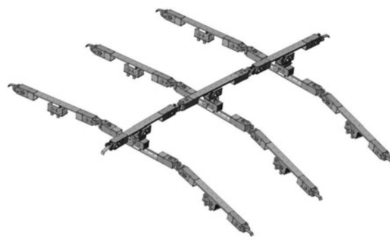
Fig. 2: The twelve link-type robots forming a six-legged robot like an insect.
