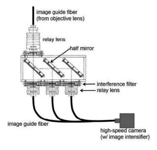
Fig. 3. Optical detection system.
