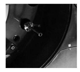
Fig. 2. Laval nozzle installed in QUEST vacuum vessel.
