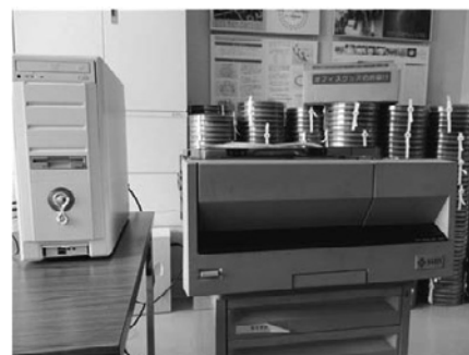
Fig. A part of the stored MT reels for Heliotron-E experimental data (top) and a set of a MT reader and PC for media conversion of the data (bottom)
