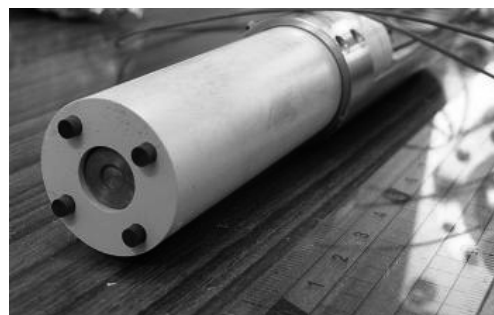
Fig. 1: Photo of the combined probe with a Cu GTP tip.
