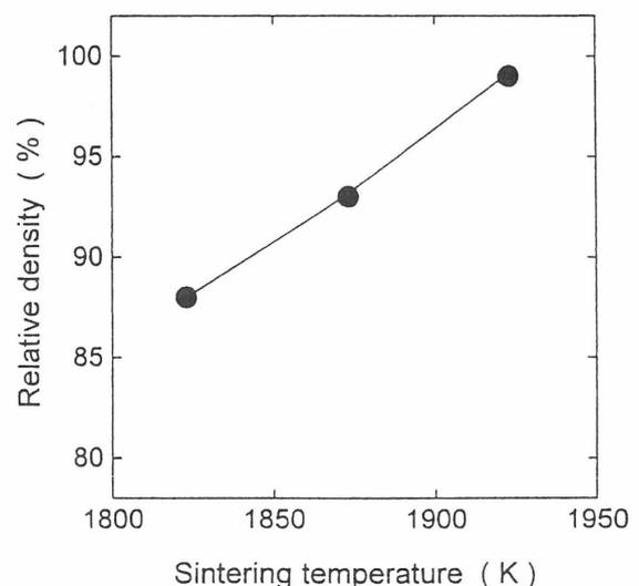
FIG. 1. Relationship between sintering temperature and relative density of the sintered bodies.
