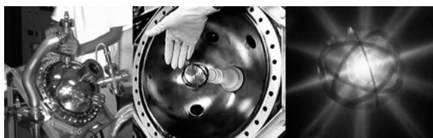
Fig. 1. A conventional glow-discharge-driven IECF device.
