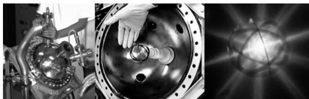
Fig. 1. A conventional glow-discharge-driven IECF device.
