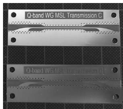
Fig. 2 PCB of 40 GHz waveguide to microstrip line transmissions.
