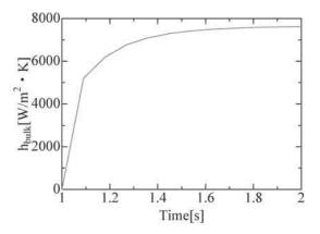
Fig.3 Trend of the bulk heat transfer coefficient (example)
