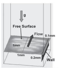
Fig. 2 Free-surface deformation due to shear flow/gravity
