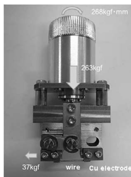
Fig.1 The conceptual design of applied uniaxial tensile strain mechanism on transport I_c measurement at 4.2K under various higher magnetic field.
