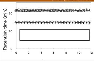
indistinguishable, independent of the concentration and repetition time. The average retention times (and relative standard deviations) were 14.8 min (1.45%), 15.0 min (0.26%), and 14.9 min (0.25%) for the protium in the 5-, 20-, and 50-cm³/1000 m³ sample gases, respectively. For deuterium they were 21.6 min (0.47%), 21.7 min (0.17%), and 21.6 min (0.22%). The difference between the protium and deuterium was about 6.5 minutes. The retention times were thus distinguishable and very stable.
