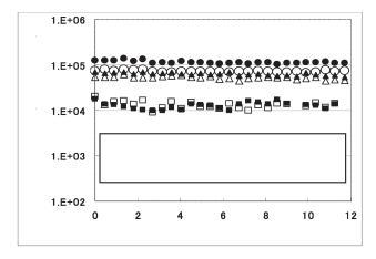
These results indicate that the peak areas obtained at the same time for both elements were stable, independent of the elapsed time and repetition time. This means that the analyzer can detect concentrations of protium and deuterium as low as about  $5~{\rm cm}^3/1000~{\rm m}^3$ .
