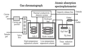
including nitrogen, contained in the sample gas. Experiments using protium and deuterium separately demonstrated that the analyzer works well regardless of differences in the hydrogen isotope. We have used the analyzer to distinguish hydrogen isotopes in three gas mixture test samples (protium and deuterium with almost equal concentrations in nitrogen). Nitrogen gas was used as the dilution gas to simulate an air sample.
