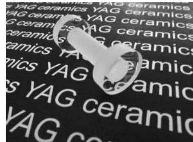
Fig.1 A photograph of the diffusion-bonded YAG ceramic sample for the measurement of dn/dT and the temperature dependence of the thermal expansion coefficient 2) .
