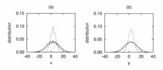
Figure 1: Evolution of distributions with a = 15, b = 1, c = 1/2,  $\omega = \pi/2$ , and  $B_{t0} = 3$  for (a) the x direction and (b) the y direction. A dash-dot line is the distribution at  $t_b = 1$  and a solid line is one at  $t_b = 5$ , where  $D_x = D_y = 10$ . A dot line is the Gaussian distribution with mean 0 and variance 100.
