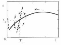
Evolution of temperature and density when density limit is reached. A case of limit cycle oscillation is shown.
