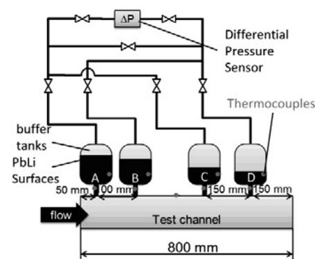
Fig. 2. Schematic view of the sub loop for differential pressure measurement
