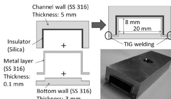
Fig. 1. Fabrication of the three-surface and multi-layer coated channel for the experiment
