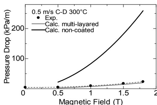
Fig. 3. Relationship between applied magnetic field and pressure drop in the region C-D with a velocity of 0.5 m/s and temperature of 300 °C
