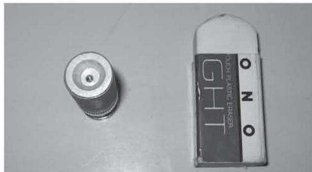
Fig. 1. Photograph of natural diamond detector. It has a size of \phi 2 mm and 0.1 mm thickness. Surface electrode is made from Au.
