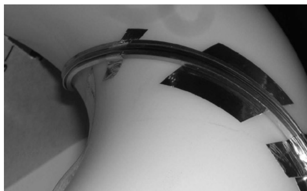
Fig. 4. The first trial of helical winding. The wire is wound in the grooves by three turns.
