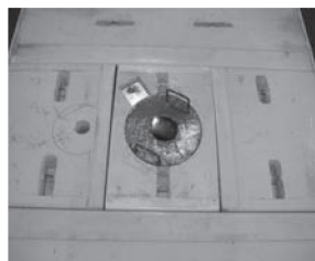
Fig.2 Exposure of IP in the experimental hole of Reactor
