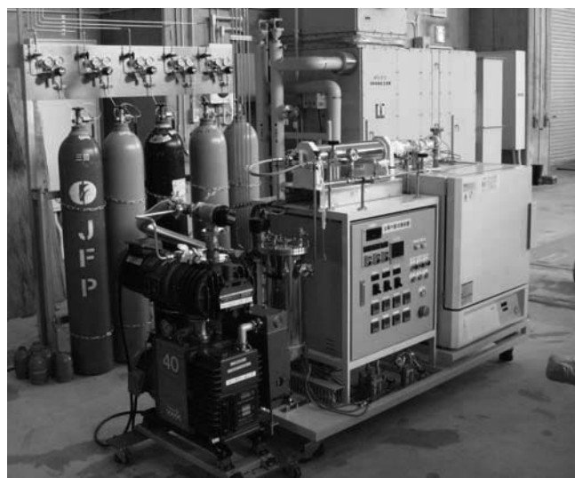
Fig.1 The photograph of the MOCVD apparatus for the large area oxide coating in NIFS.
