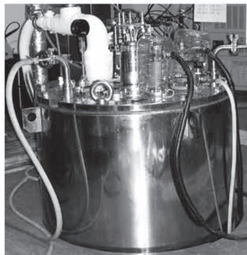
Fig.1 18T class High-Field Superconducting Magnet in Tsukuba Magnet Laboratory of National Institute for Materials Science (TML-NIMS)
