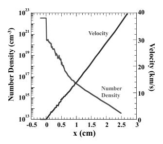
Fig. 2 Number density and velocity profiles of lead.
