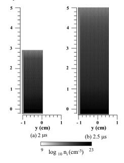
Fig. 3 Particle number density profiles obtained by 2dimensional simulation
