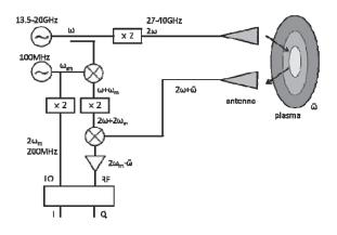
Fig. 3 Improved reflectometer system for density fluctuation measurement
