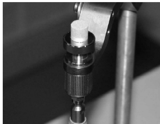
Fig. 1. Appearance of coaxial cable probe and metal powder compact sample.
