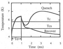
Fig. 2 Time variation of calculated conductor temperature at the center of disturbane
