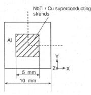
Fig.1 Cross-section of model conductor
