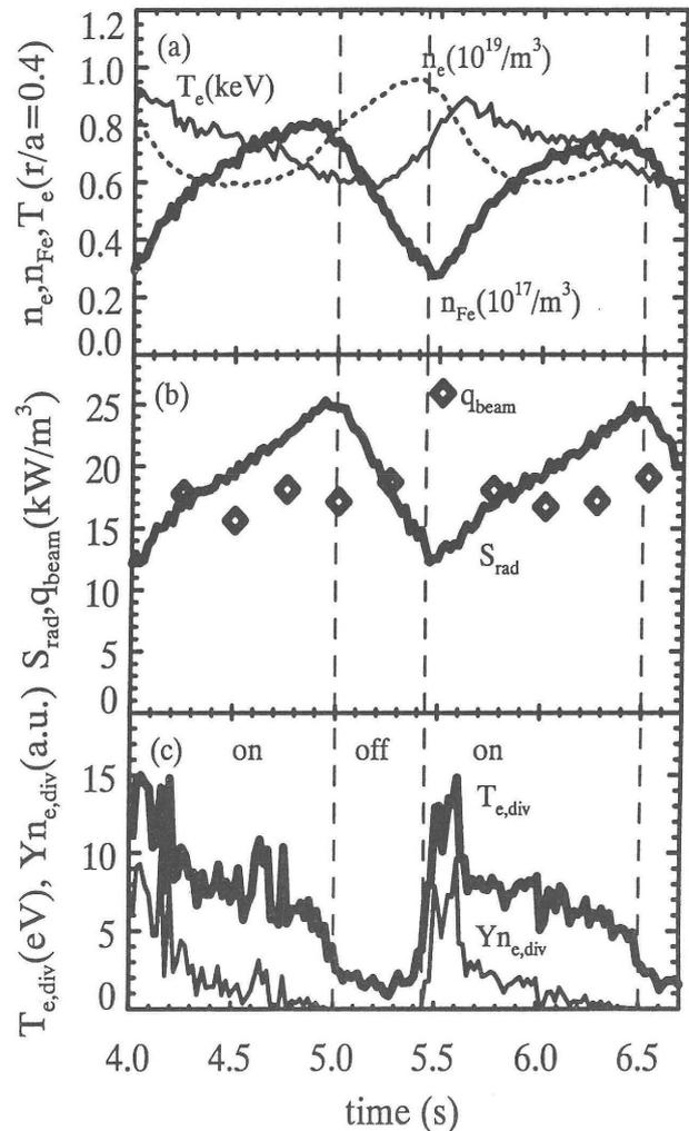
Figure 1 Evolution of (a) measured electron density and temperature, calculated iron density, and (b) measured radiation emissivity, beam deposition power density at  $\rho = 0.4$  and (c) the measured electron temperature at the divertor and the calculated sputtering yield, during shot #6690.
