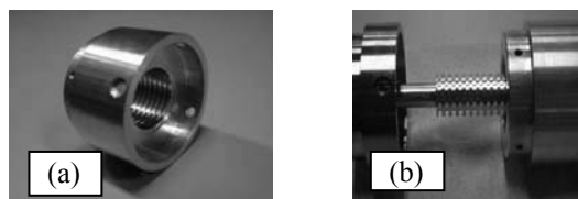
Fig.3 Periodically corrugated cavity; (a) corrugated hollow waveguide and (b) corrugated inner conductor.
