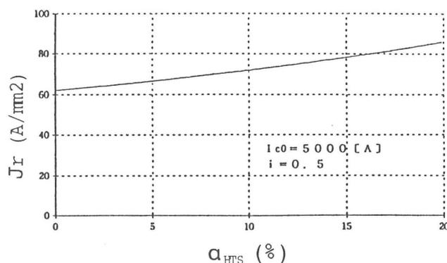
Fig. 1 Dependency of stabilized current density on  $\alpha_{HTS}$ .
