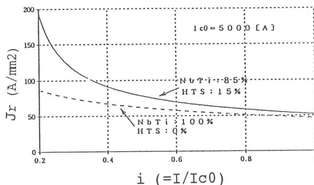
Fig. 2 Dependency of stabilized current density on  $i$ .
