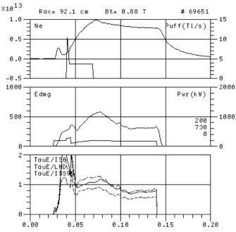
Fig. 2. NBI discharge with deuterium gas puff
