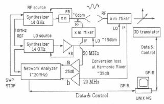
Fig.2 : Low Power Test System
