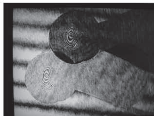
Fig. 5 Interference pattern of foam shell filled with liquid hydrogen, indicating uniform distribution of liquid hydrogen.
