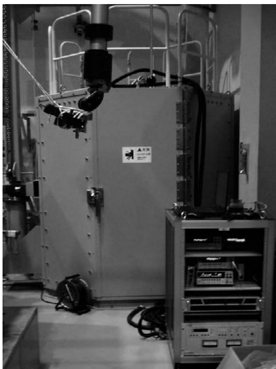
Fig. 1. Magnetic field shield structure (back) and control and data acquisition system (this side).
