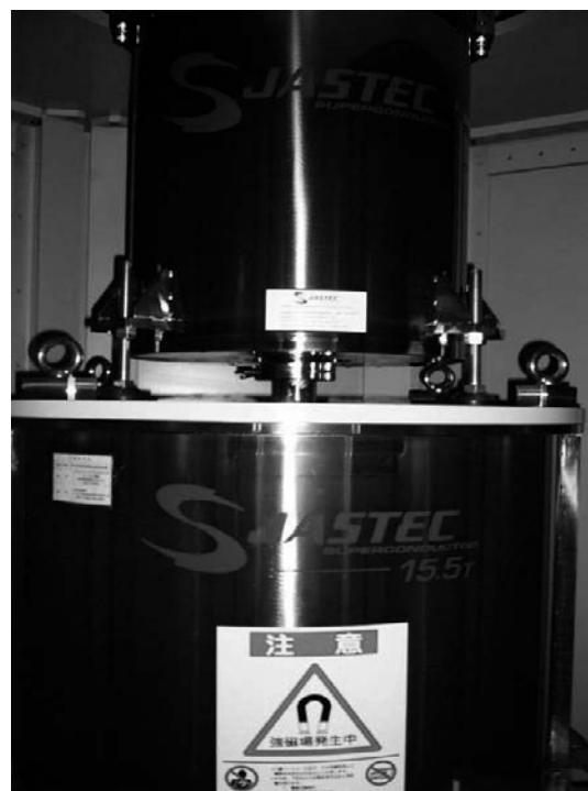
Fig. 2. 15.5 T superconducting magnet (lower) and variable temperature insert (upper) in magnetic field shield structure.
