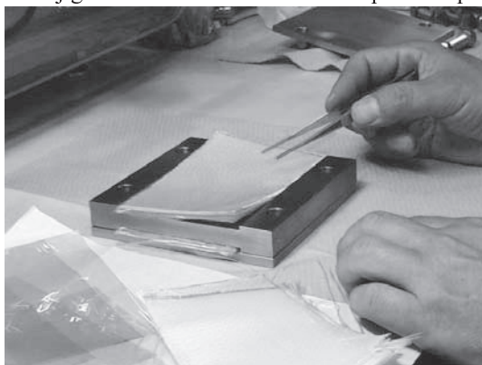
Fig. 1. Laminate process of polyimide film and glass cloth in the mold jig.
