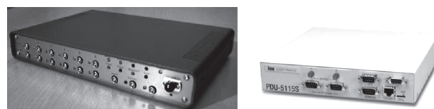
Fig. 3 New FPGA-based timing demodulator (left) and remote power controller (right) boxes: From the 10 th LHD campaign, they have been ready for distribution. They can help us to reduce both the new installation and human maintenance costs for plasma diagnostics.
