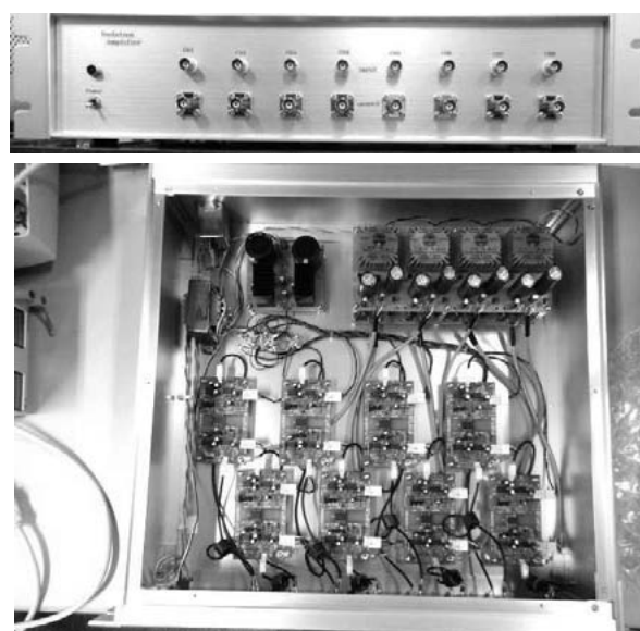
Fig. 2 Front and inside photos of the new 8-channel isolation amplifier: Primary-side power supply is independently implemented for each channel, whereas the secondary-side one is shared with a common (chassis) ground.
