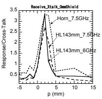
Fig. 3 Ratio of the response and the cross-talk in DLDA with shield as a function of distance (p) between the shield and the dipole.
