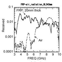
Fig.2 Frequency response of dipole antenna with/without the dielectric lamination.
