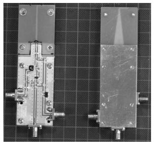
Fig. 1 Dielectric Laminated Dipole Antenna (DLDA).
