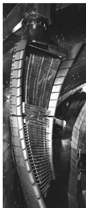
Fig. 1 ICRF antennas with and without Faraday shield in LHD in 2013
