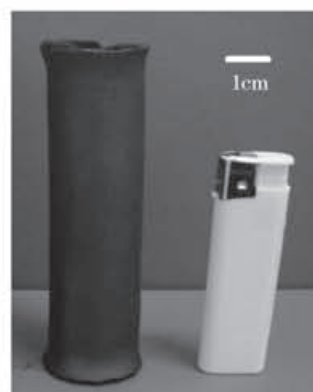
Fig. 1 Prepared large size Bi-2223 bulk composed with meshes
